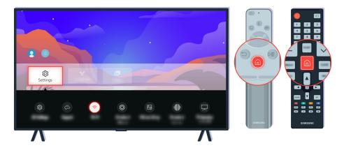
If your TV is connected to the network, you can set it to receive periodic updates automatically. On the remote control, press the a button and move to  $\equiv$  Menu  $\Rightarrow$  s Settings  $\Rightarrow$  Support using the directional button.
