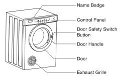
The exhaust grille has a range of positions, which allows you to select the optimum exhaust air angle. Simply hold the grille and rotate it until it hits the built-in stop.
